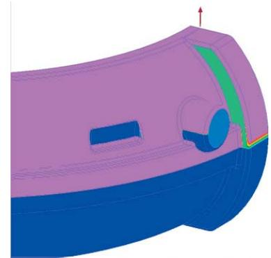
Draft analysis showing undercut areas. Dark blue indicates undercut areas requiring design concession, loose pieces or cores.
